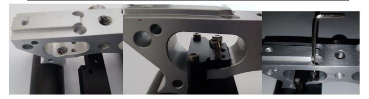
Please note that you must remove the tripod adapter plate of the 1.2m track first, in order to access the mounting spot.
