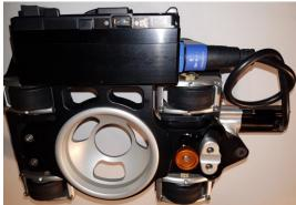
Do not connect neither the motor cable nor the DynaStick cable to the RF side (antenna side) - center picture. Besides that the cables won't fit, the connectors on there are for other purposes!
